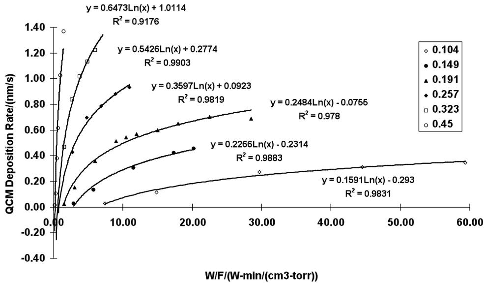
**Figure 4.** Linear fit of  $A_i$  and  $b_i$  terms from the equations shown in Figure 3 for the equations  $Y = A_i \cdot \ln(X) + b_i$ .
